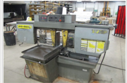
HYD-MECH S-23P HORIZ. BANDSAW WITH MITER CUT
