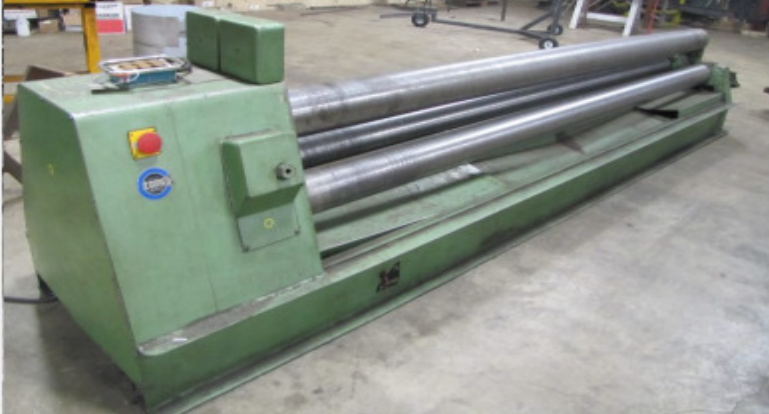
ROUND O MODEL PS 205 14' X 3/16" PLATE ROLL, AIR DROP END, MFG. 1983
