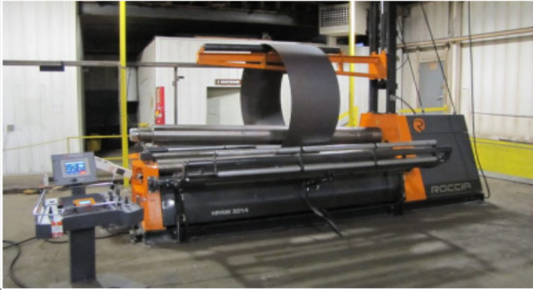
2013 ROCCIA MODEL HR4W 10' x 1/2" 4 ROLL PROGRAMMABLE PLATE BENDING ROLL
