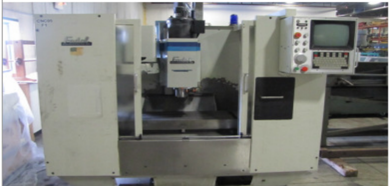
1988 FADAL VMC 40, FADAL 88 CONTROL, TRV. X-22, Y-16", Z-20", 20 ATC. SPINDLE TAPER CAT 40
