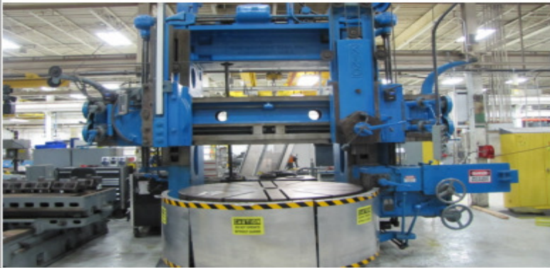
72" KING VBM, FLUSH FLOOR, 4-JAWS, RAM, TURRET, SIDEHEAD POWER RAIL, MAX RPM 45.5 VARIABLE, PENDANT CONT. DRO
