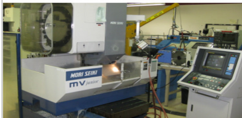
1992 MORI SEIKI MV-JR VMC, FANUC 0-M CONT. WIRED FOR 4TH AXIS, TRV. X-22", Y-16", Z-18", 8K SPDL., 20 ATC, CAT 40
