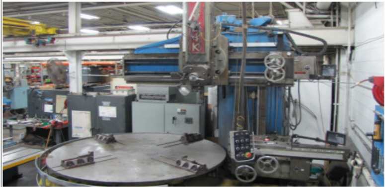
50" / 92" HAVLIK VBM, FLUSH FLOOR, SLIDING TABLE, TURRET, SIDEHEAD, MAX RPM'S 120 VARIABLE, 4-JAWS, MAX. HEIGHT 42" DRO
