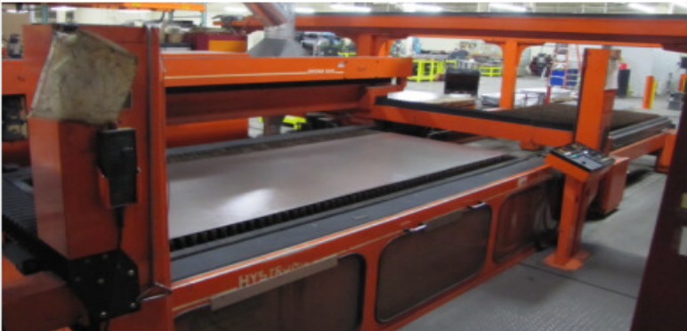
BYSTRONIC BYSTAR 3015 FLYING OPTIC 2800 WATT LASER, BYSTRONIC CONT., DOS 6, SHEET SIZE 5' X 10', LOAD /UNLOAD
