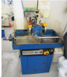
AGATHON 175-DIA PRECISION TOOL GRINDER, WHEEL DIA. 6.89", MAX SPEED 2700 RPM
