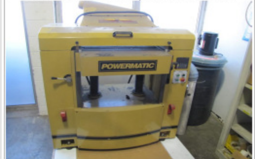
2014 POWERMATIC WP2510 PLANNER, HELICAL CUTTERHEAD, MAX. WIDTH 25", MAX. THICKNESS 9", DEPTH CUT 1/4"
