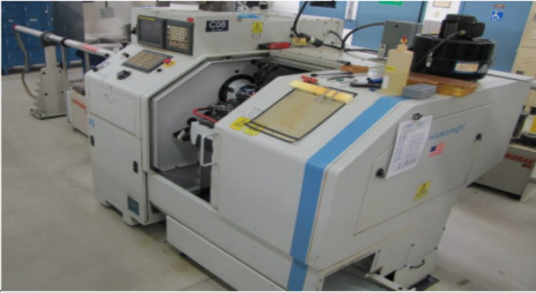
2004 HARDINGE QUEST GT27SP GANG TYPE CNC, GE FANUC 21i-TB, 5C COLLET SPDL, RHINO BAR FEED
