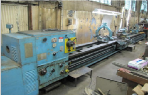
37" x 314" WMW NILES DLZ 800 III LATHE, SWING OVER CARRIAGE 24", IN / MM THREADING, 25" 3-JAW, STEADY REST
