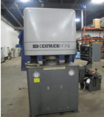
EXTRUDE HONE VECTOR 8/6 ABRASIVE FLOW MACHINE, A&B CONT., 8" MEDIA CYL., 6" HYD. CYL.
