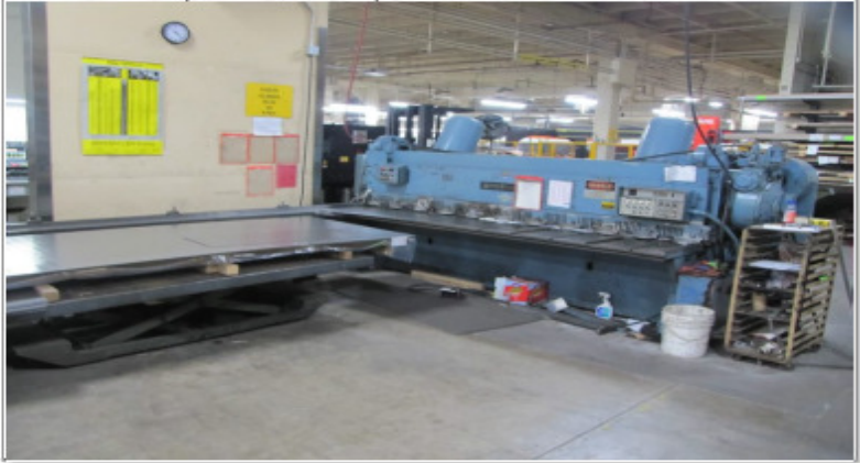
CINCINNATI 2CC10, 1/4" X 10' MECH. SHEAR, 36" FOPBG, 10' SQ. ARM, REAR SHEET CONVEYOR
