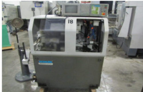
NOMURA NN-13SII CNC SWISS TYPE AUTOMATIC TURNING MACHINE, MITSUBISHI CONT., LIVE TOOLING
