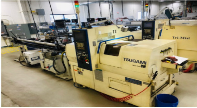
2007 TSUGAMI BW12-III 7 AXIS SWISS TYPE AUTOMATIC SCREW MACHINES WITH LNS BAR FEED, 2 AVAILABLE
