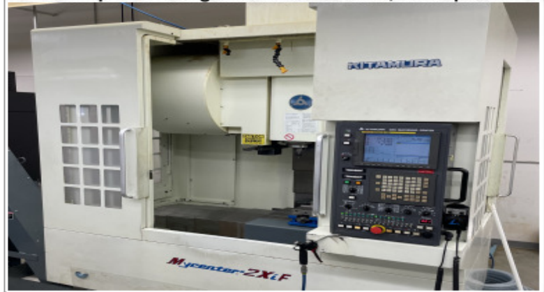
2005 Kitamura Mycenter 2XiF, 4th Axis, VMC-Fanuc16iMB, Thru Spindle & High Pressure Coolant, 20K Spindle
