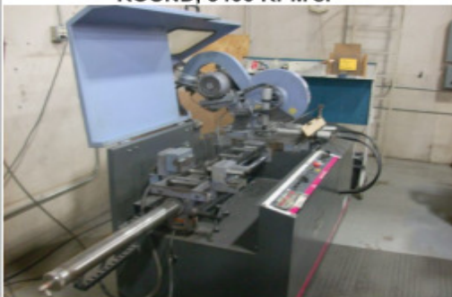
14" DAKE/MEP Cobra 350 AX Non-FERRIS AUTOMATIC COLD SAW, CAPACITY 4.5" ROUND, 3400 RPM's.
