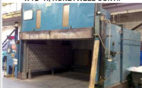
INFERATROL WALK IN OVEN, MAX TEMP. 240F SOLVENT RATED (500 F CONSTRUCTION) SIZE 138" W X 126" L X 72" H, HONEYWELL CONT..
