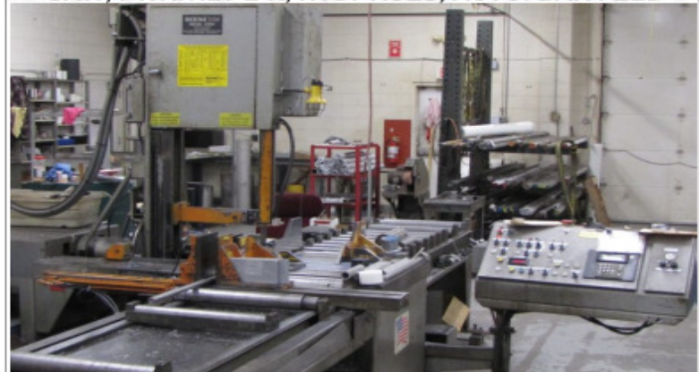
1997 HEM V120HA 18" x 24" VERT. PROGRAMMABLE SAW, PWR. TILT L-R, HYD. VISES, AUTO. BAR FEED
