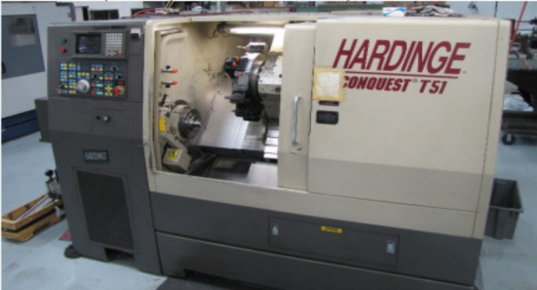
1995 HARDINGE CONQUEST T-51 CNC LATHE, C-AXIS, LIVE TOOLING, GE FANUC 18A CONT. TAILSTOCK
