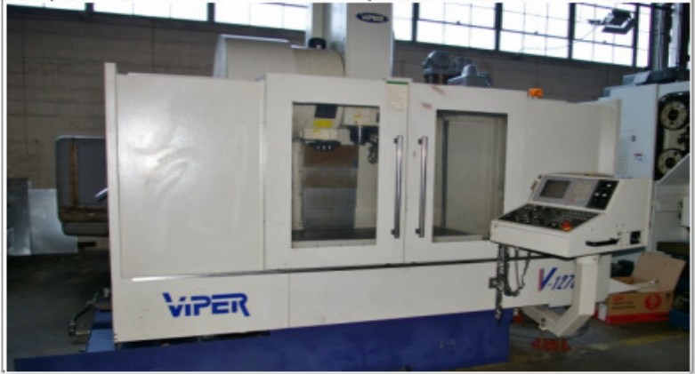
2003 MIGHTY VIPER VMC1270A MITS. MAGIC 64, TABLE 54" X 23.5" 20 ATC, 4TH & 5TH AXIS READY
