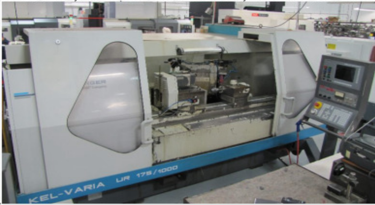
1997 KELLENBERGER UR 14" x 40" CNC UNIV. CYL. GRINDER, KELCO 90 CONT. B AXIS, ID ATTACHMENT
