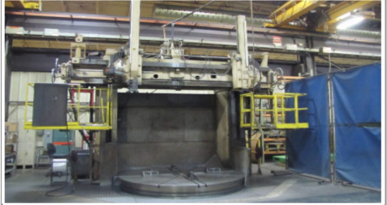
Cincinnati Hypro 120" VBM, 4-Jaw Chk, Approx. Trv. 103" UR, 96" UT, Rams: Left 70", Rt. 50", DRO's
