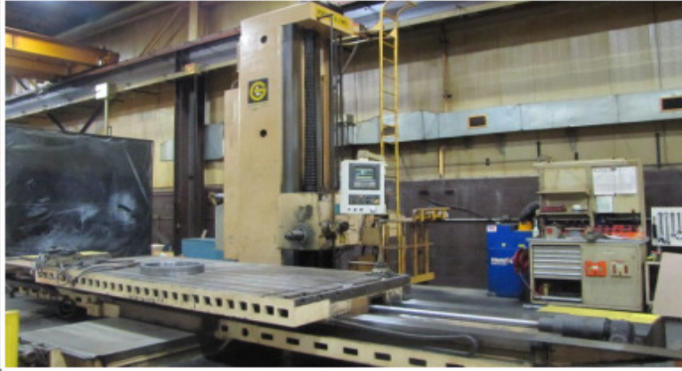
Giddings & Lewis 6" CNC HBM, A/B 9 Ser. Cont., X-140", Y-140", Saddle 60", Quill 30", 50 Taper, Prog. Rotary Table.
