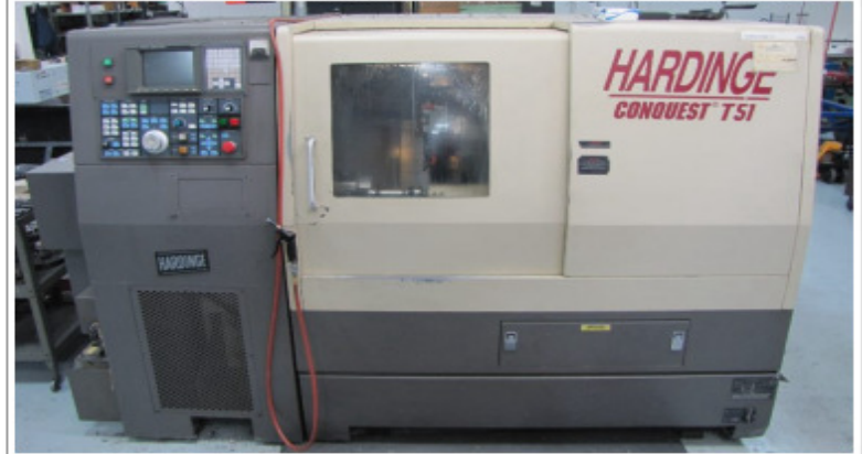
Hardinge Conquest T-51 CNC Lathe, GE-FANUC 18-T, Chk Cap. 10", Turn Dist. 22", Bar Cap. 2", 12 Sta. Turret
