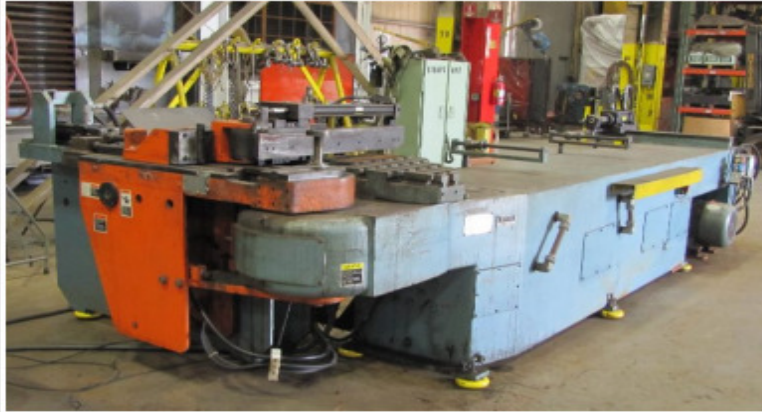
PINES #4 Hyd. Tube Bender, Magelis Prog. Cont., Max Bending Angle 180 deg., Capacity: 6" OD X .250 Wall
