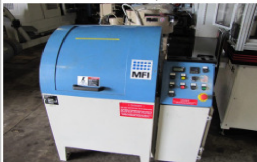
MASS Finishing (MFI) HZ-40 Barrel Finishing Machine, Mfg. 2012, Barrel Dia. 12-3/4" L X 6-7/8" W, 4 Barrels
