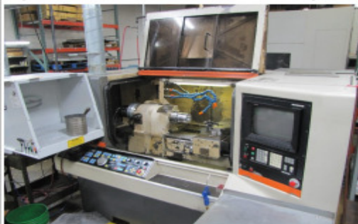
Hardinge CHNCII+ SP CNC Lathe, Fanuc 10TF, 14" Swing, 16C Collet Cap., 1-7/8" Spdl Hole, 8 Sta. Turret, Max 5000 Rpm's
