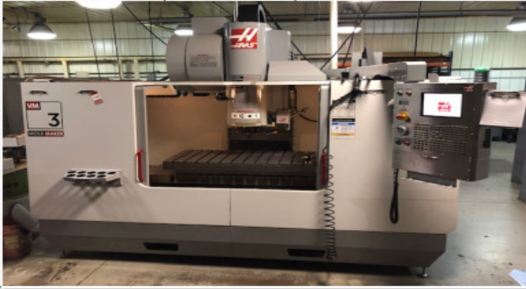
2004 HAAS VM-3 MOLDMAKER, 24 ATC, CAT 40, TOOL SETTING PROBE, CHIP AUGER, ONE OWNER MACHINE
