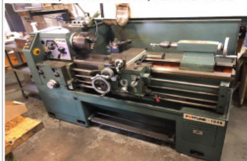
FORTUNE 1640 ENGINE LATHE, DRO, 16" x 40", IN/MM THREAD, 2" SPINDLE BORE, 3-JAW CHUCK, ALORIS TOOL
