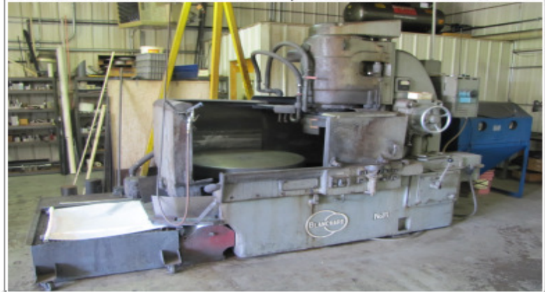
BLANCHARD NO. 18 ROTARY SURFACE GRINDER, APPROX. 3/8" CHUCK LIFE, EXTERNAL COOLANT
