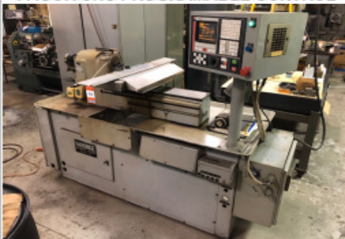
HARDINGE/AHC LATHE WITH RETROFITTED FAGOR CNC PROGRAMMABLE CONTROL
