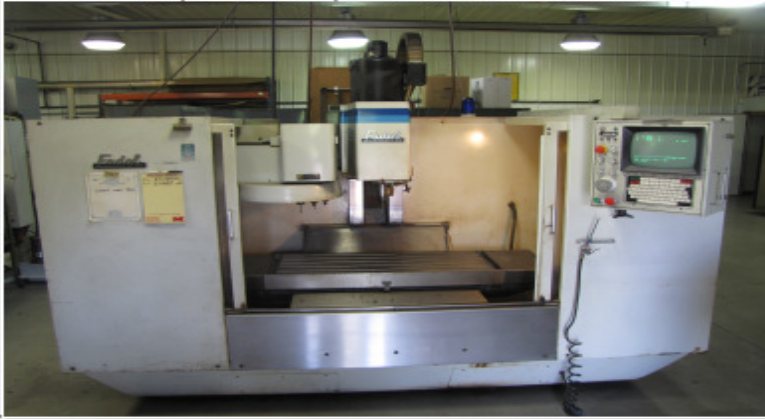
FADAL 4020HT VMC, 21 ATC, CAT 40, RIDGID TAP, COOLANT, ONE OWNER MACHINE
