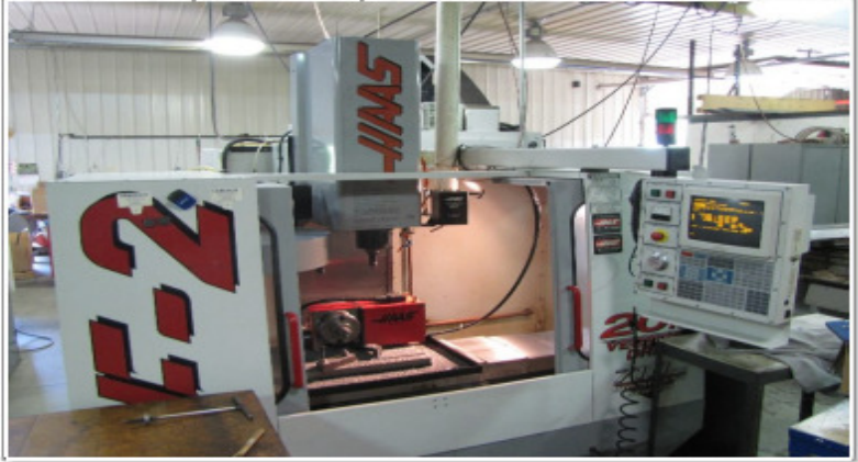
1998 HAAS VF-2 VMC, 20 ATC, CAT 40, CHIP AUGER, 20HP, COOLANT, ONE OWNER MACHINE
