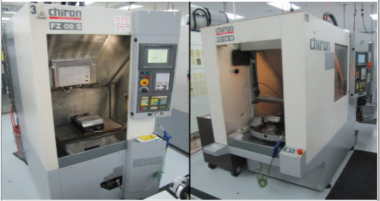
CHIRON FZ 08 W & FZ 08 S VMC, GE FANUC 21 CTRL'S, 12 ATC, HSK 32 SPINDLE TAPER, BOTH MFG. 1997
