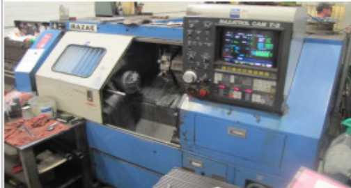
MAZAK QT10N UNIV. CNC LATHE, CAM T-2 CTRL, 8 STATION TURRET, TAILSTOCK
