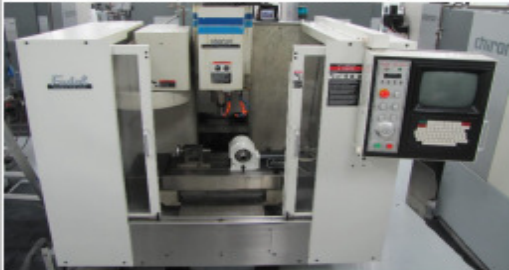
FADAL VMC 15 4TH AXIS VMC W/ INDEXER & TAILSTOCK, FADAL HS88 CRTL, 1995
