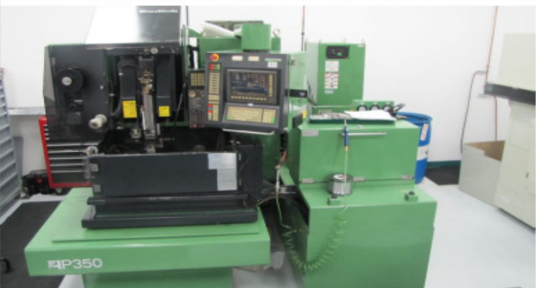
SODICK AP350 CNC WIRE EDM, MARK 25 CTRL, TVL'S X-13.7", Y-9.8", Z-8.6", AUTO THREAD, SUB-MACHINING
