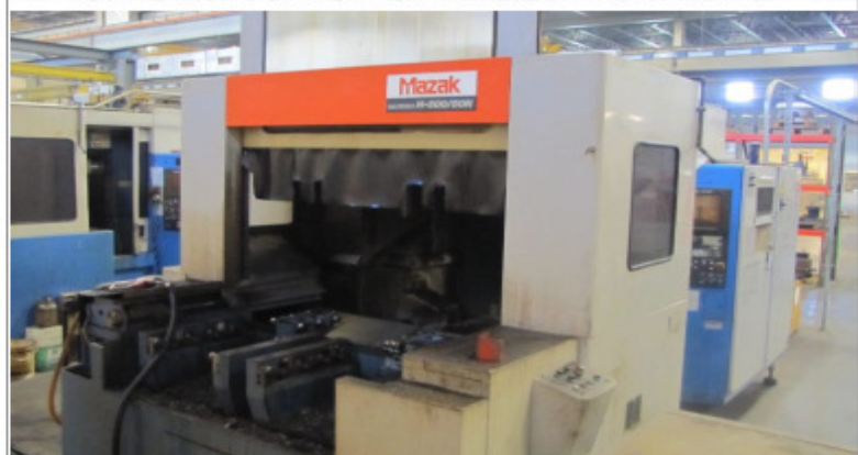
MAZAK 1993 H-500/50N & 1991 H-500/50 2-PALLET HMC, MAZATROL M-32 CTRL'S, 19.7" X 19.7" PALLETS, TSC, 1 DEG., 120 ATC
