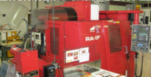
MATSUURA MODEL RA-1F 2-PALLET VMC WITH 4TH AXIS ROTARY INDEXER, MFG 1992
