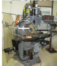
BRIDGEPORT SERIES I EZ-TRAK SX 3-AXIS CNC VERTICAL MILL, MFG 1992
