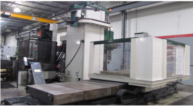
KURAKI KBT-13DXA 5.12" HBM, GE FANUC 15M X-118", Y-78", 63" x 70" TABLE, 1 DEG. INDEX, 1993
