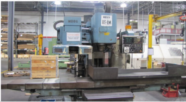
Ooya RE-1M VMC, FANUC 6M, X-55", Y-15", Z-20" 18.5" X 63" TABLE, 20 ATC, CAT 40 TAPER, 4K SPDL.
