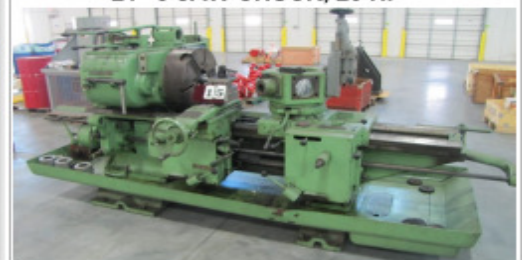
WARNER & SWASEY 3-A TURRET LATHE, 23" X 59" CAPACITY, 4.5" BAR CAP., 21" 3-JAW CHUCK, 20 HP
