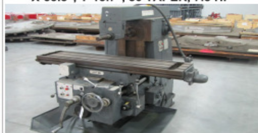
CINCINNATI MILACRON 207MK HORIZ. MILL, 13.750" X 59.5" TABLE, X-33.5", Y-13.7", 50 TAPER, 7.5 HP
