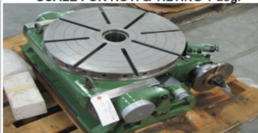
NIKKEN NST-500HP 20" MANUAL UNIVER. ROTARY TILTING TABLE, SCALE FOR ROT. & TILTING 1 deg.
