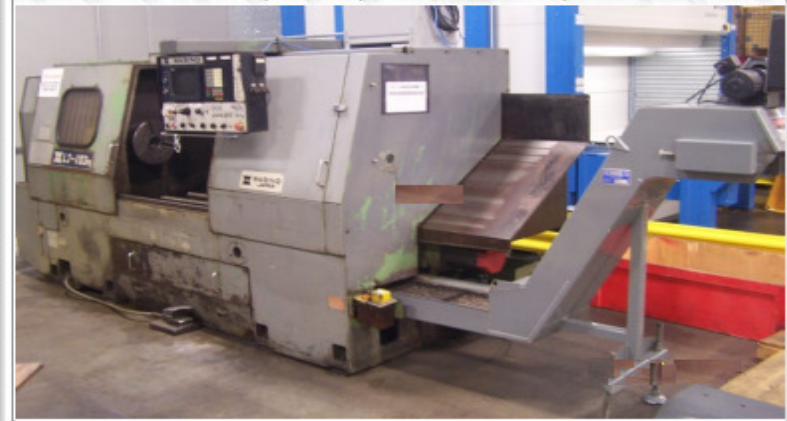
WASINO LJ-103M TURNING CENTER FANUC 10T LIVE MILLING, C-AXIS, 12 STA. TURRET, 12" 3-JAW
