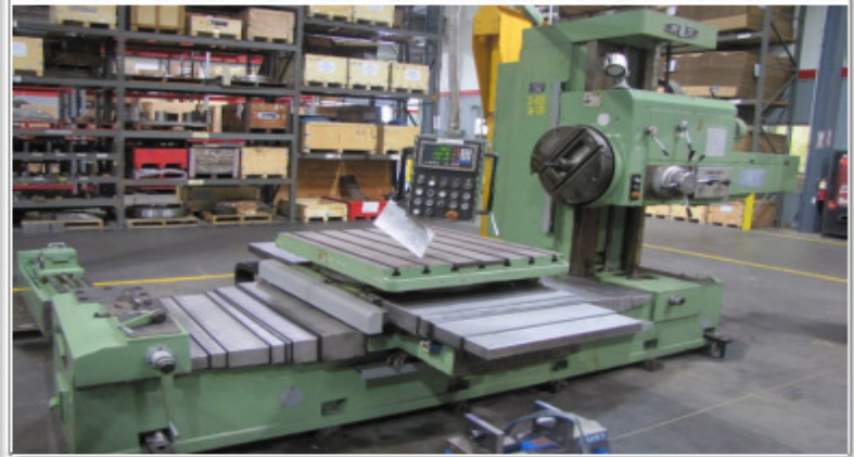
SHENYANG 4.3" TPX6111B HBM, X-36", Y-36", Z-56" 44" X 38.5" TABLE, FACING HEAD, OUTBOARD, 2008
