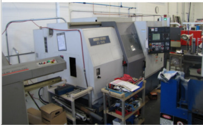
MORI SEIKI ZL-150 SMC TWIN TURRET CNC LATHE, SUB-SPINDLE, LIVE TOOLING, C-AXIS, SMW BAR FEED, 2000
