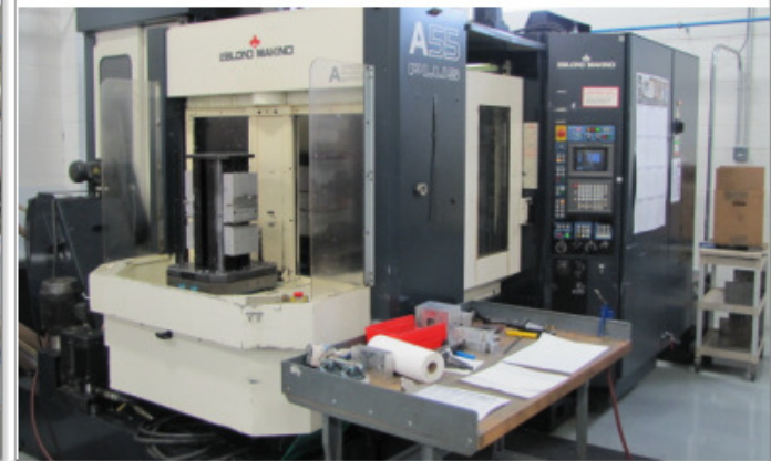
LEBLOND MAKINO A55 PLUS HMC, PRO 3 CNC CTRL, 128 POS. ATC, THRU SPINDLE COOLANT, CAT 40, 20K RPM
