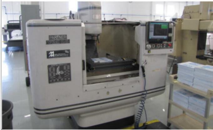
MILLTRONICS VM-16 WITH CENTURION 6 CTRL, 16" X 45" TABLE, 12 POS. ATC, CAT 40, 6K RPM, 1997
