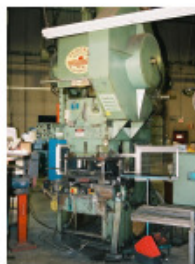
FEDERAL 110 TON OBI B.G. PUNCH PRESS 5" STR. 40 SPM, 42" X 27" BED, AIR CLUTCH, 1977
