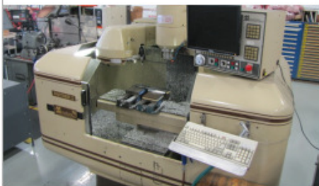
MILLTRONICS P1 VMC, 12 POS. ATC, CAT 40, 6K RPM, USB PORT
