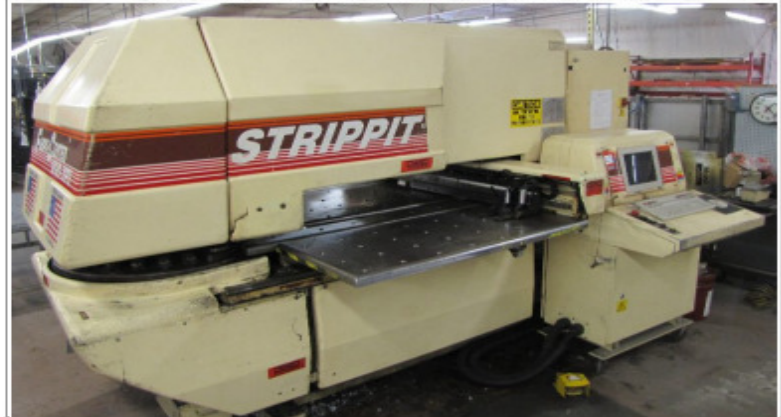
1995 STRIPPIT MODEL FC 1000XP II 20.5MT CNC TURRET STRIPPIT PC CONT. 3-AI, AUTO REPO. 20 STA
