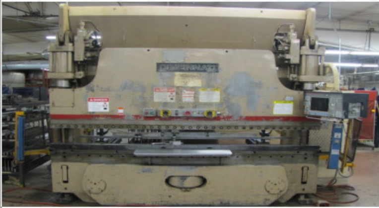
1989 CINCINNATI MODEL 175 AF HYD. 175 TON X 12' PRESS BRAKE, AUTOFORM CONT. 24" BG, CROWNING.
