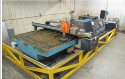
LOCKFORMER VULCAN 2900 PLAZMA CUTTER, 5' x 10' DOWN DRAFT TABLE, A&B CONT. HYPERHERN MAX 100.
