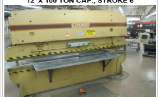
1992 STANDARD AB 100-12 HYDRAULIC PRESS BRAKE, w/ AUTOMECH AUTOGAUGE CNC 2000 BACK GAUGE, 12' X 100 TON CAP., STROKE 6"
