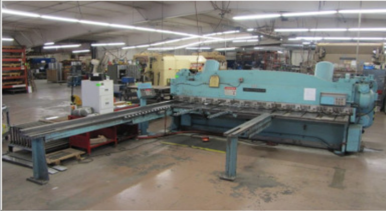
1990 CINCINNATI MODEL 20C12 PWR/ SQ SHEAR, PROG. CONT. FRONT GAUGING, 36" FOPBG. SCRAP CONV.
