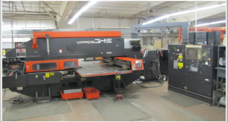
1994 AMADA MODEL VIPROS 345 CNC 33 TON TURRET PUNCH, FANUC 04PC, 2-AI, AUTO REPO, 58 STA. TURRET
