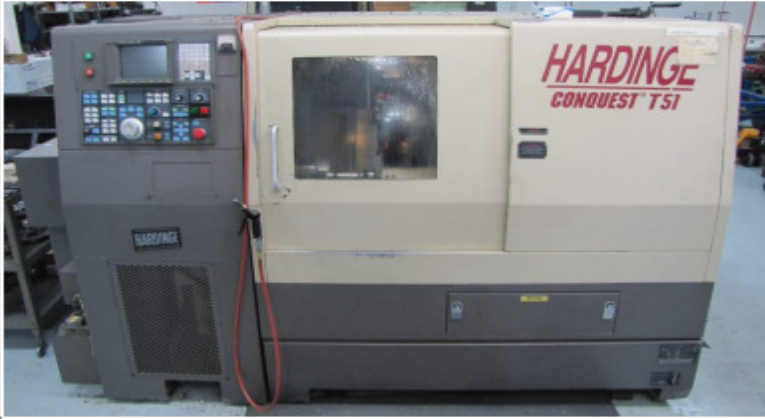
HARDINGE Conquest T51 CNC Turning Center, Fanuc 18T, Max. Swing 26", Prog. Tailstock, Tool presetter 1997
