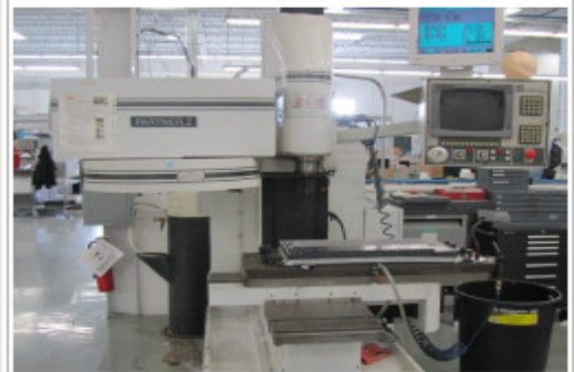
Milltronics Partner I CNC VMC, Centurion V Cont., Table 16" X 45", TRV. X-30", Y-16", Z-20", 20 ATC, Taper 40, 5K Spindle
