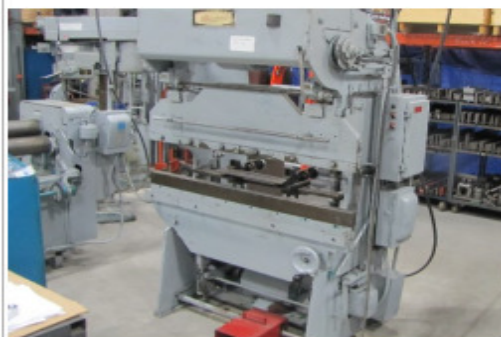
DiAcro 17 Ton X 4" Hyd.-Mech. Press Brake, Capacity 4' X 14ga., Ram Strk. 2" Dual Speed, FOPBG.
