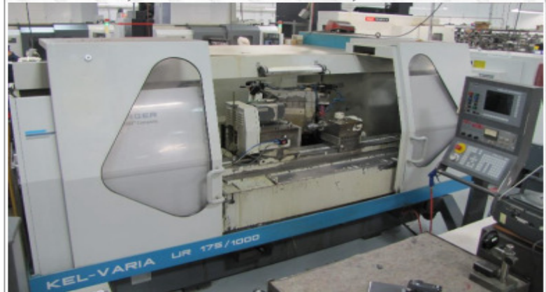
1997 KELLENBERGER UR 14"x 40" CNC UNIV. CYL. GRINDER, KELCO 90 CONT. B AXIS, ID ATTACHMENT
