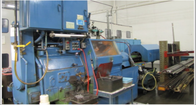
2-ACME-GRIDLEY Model RA-6 1-1/4" 6 Spindle ASM's, THREADING & REAMING, STOCK STAND & REEL
