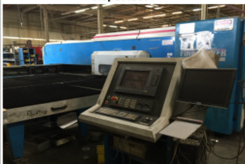
FINN Power F6-25-SB-30 CNC Turret Punch 30 Ton, Siemens 840D Cont., Max Sheet: 122" X 61", 8-Auto Index, Sheet Repo.1997
