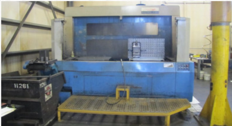
Mazak H-800 Twin Pallet HMC, 31.5" X 31.5" Pallets, M-32, B-Axis, CTS, 40 ATC, ALSO: H-400N HMC, CTS
