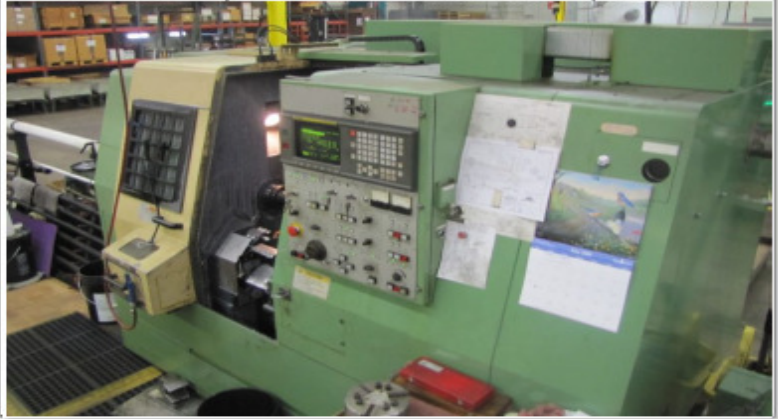
MORI SEIKI ZL-15S CNC LATHE WITH MF-D6 CONT., SUB-SPINDLE, 12 & 8 STATION TURRETS, BARFEED
