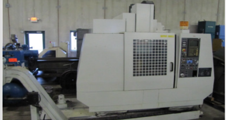
MATSUURA MC800 VF VMC WITH YASNAC i80 CONT. 16" X 45" T-SLOTTED TABLE, 40 TAPER MFG. 1997
