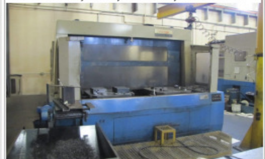
MAZAK H-800 HMC WITH MAZATROL M-32 CONT. 31.5 x 31.5 PALLET, 50 TAPER, CTS, 40 ATC, MFG 1989
